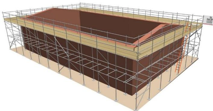
*Figure 4. A typical scaffold design*
